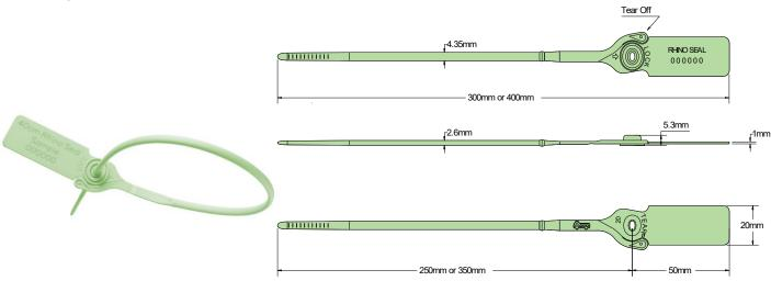
The Acme **RHINO Seal** is a smooth ribbon, pull-tight seal manufactured from Polypropylene material. The design profile is unique and features rolled heat staking technology to secure the metal spring insert to the body, thus providing clear evidence of tampering if forced open or cut. The seal is manufactured with tear off tag. The excellent breaking strength, combined with a ribbon width of less than 5mm, makes this seal the ideal choice for many applications.
