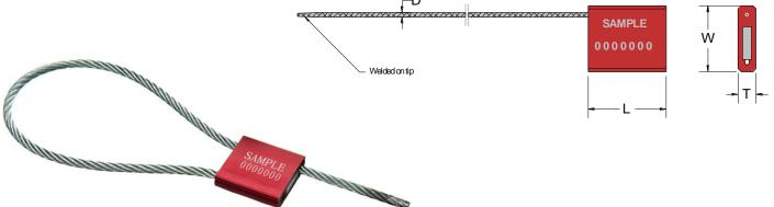
The Acme **CS1 Cable Seal** is available in various cable lengths and diameters to suit all requirements. The lock body is manufactured from die-cast aluminum and the cable from non-preformed galvanized steel. The cable has a welded tip for ease of locking and should the cable be cut it unravels making it impossible to re-lock the seal again without showing obvious signs of tampering. The cable seal require cutters for removal.
