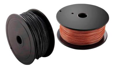
The Acme **Sealing Wire** is available in galvanized steel, copper and stainless steel and can be supplied on plastic spools or in cut lengths. The wire consists of a centre core wire and an outer wire, which is spirally lashed around the inner core wire providing an excellent thread type grip to prevent slippage or removal after the seal has been compressed.
