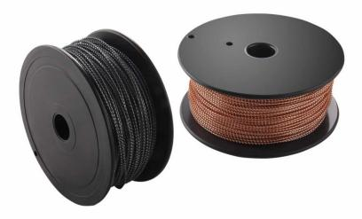
Acme **Sealing Wire** is available in galvanized steel, copper and stainless steel and can be supplied on plastic spools or in cut lengths. The wire consists of a centre core wire and an outer wire, which is spirally lashed around the inner core wire providing an excellent thread type grip to prevent slippage or removal after the seal has been compressed.
