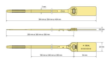
The Acme **H Seal** is a smooth ribbon, pull-tight seal manufactured from Polypropylene material. The design features rolled heat staking technology to secure the metal spring insert to the body, which provides clear evidence of tampering if forced open or cut. The seal can be manufactured with or without gripping spikes and label tag if required. This seal is suitable for many applications where strength is the requirement.
