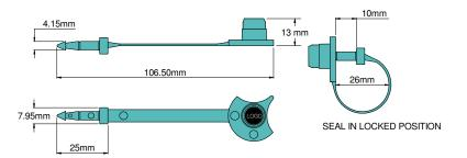
The Acme **G Lock Seal** offers a cost effective solution for the sealing of garment bags in transit or storage. It is manufactured in Acetyl material and can be supplied plain or sequentially numbered. The seal can be supplied with a different colour cap for easy identification, with or without a company logo. The design incorporates a grooved break-off point for easy removal.
